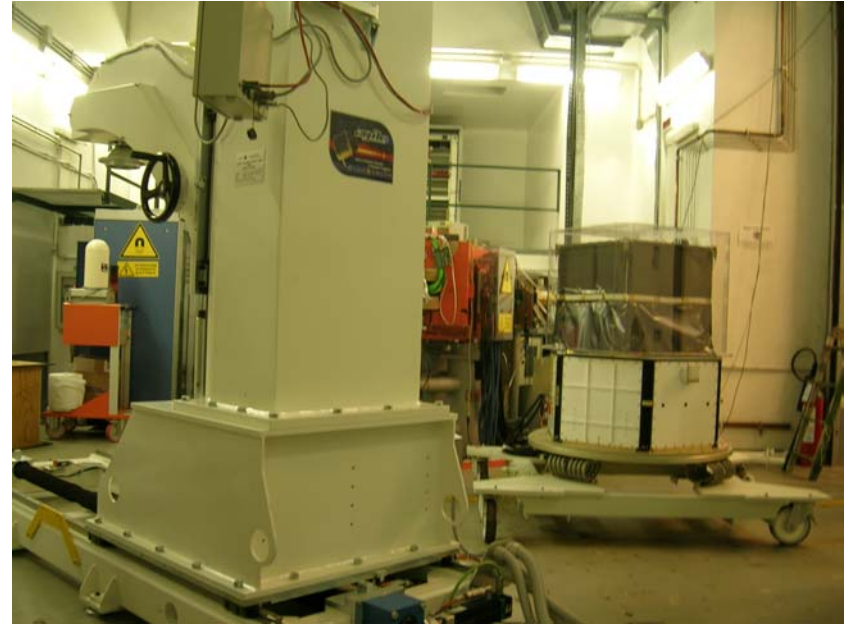
AGILE IPL on its transportation trolley is ready to be mounted on Calibration MGSE positioned in front of the Beam
